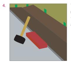
Tap the joint with the rubber mallet using a downward angle striking motion towards the adjoining end joint until the tongue and groove lock together on the side and ends.
