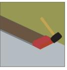
The end joints of this product features an integrated click-locking system with pushdown technology for an easy and speedy installation. Align the tongue and groove on the end joint of the next piece and press down. As the panel reaches is final position, the tongue flexes back and into the wedge groove on the folded panel,
