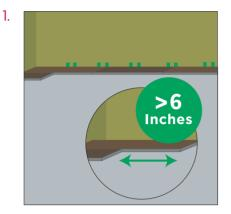
For tile installations, begin the second row with a half tile. For plank installations, if the cut plank is at least 6" in length, use it to begin the second row. If the cut plank is shorter than 6" do not use it. Instead, begin with a new board that is at least 6" in length and allows 6" between the end joints on the adjacent planks. End joint spacing for tiles should always be equal to a half tile.
