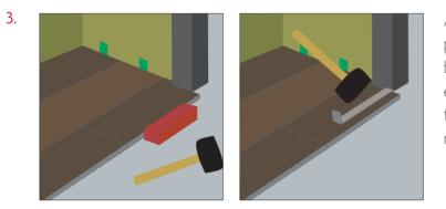
After the groove ledge has been trimmed, place the board in place and tighten with a pull bar. The installer must be sure that the required expansion gap has been maintained and the flooring is not pinched.
