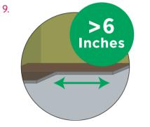
Maintain proper spacing (at least 6" for planks, and equal to half its length for tiles) between end joints for best appearance.
